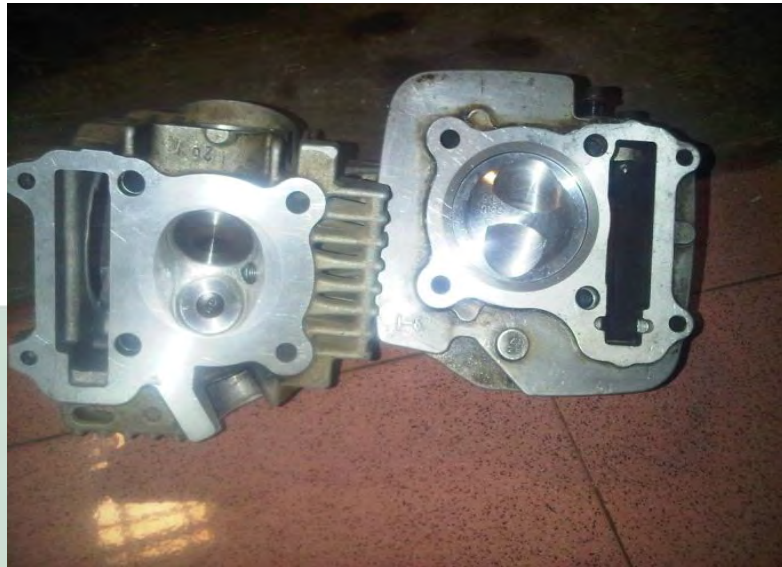
Figure 4.1 (cylinder head + cylinder blok dengan isi piston, valve, and ring valve 150cc)
